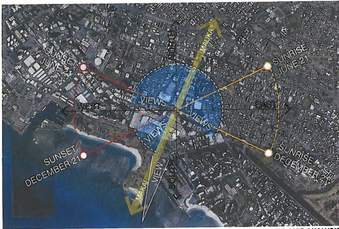
VIEW, SOLAR, AND AXIS ANALYSIS
