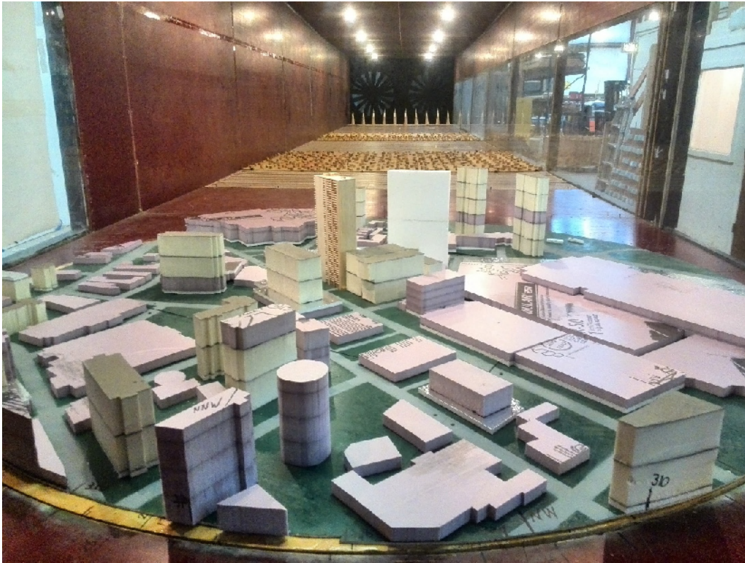
Wind study model, from another Honolulu project, viewed from northwest looking upwind into the wind tunnel. Upwind of the test section can be seen the devices used to simulate surface conditions beyond the detailed model.
